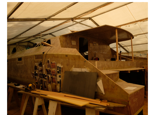
Rohbau Katamar Ocean Youth Sailing
